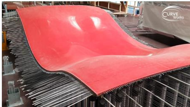
Curve Works adaptive mould "Bee" is 2.5 x 1.3 m. used for higher curvature parts. ©CURVE WORKS
