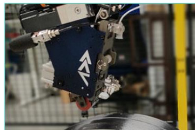
Robotic automatic tape placement ©10XL
