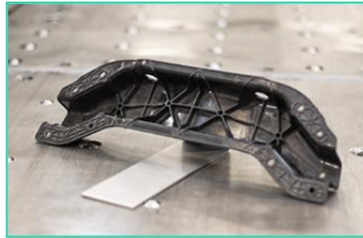
Hot stamped and over-injected part ©INEGI
