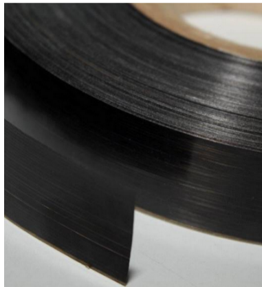
Figure 5. Composite material prepreg. PA6 matrix-based
